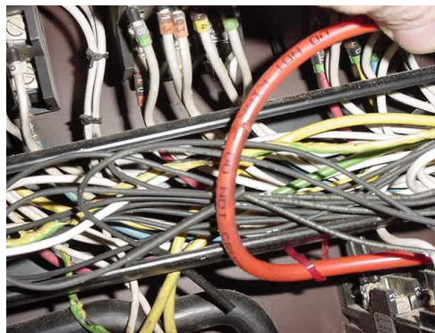
Above: Burst tube following overheated cable
