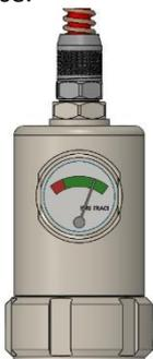
Remove the filling adapter and thread the pressure gauge & o-ring into its place to verify that the tubing is pressurised to 12bar (174psi) (pressure may have to be adjusted for temperatures higher or lower than 20°C (68°F)).
